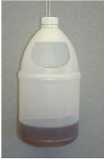
A Jug Trap, sometimes referred to as a Sugar-Bait Trap, is a plastic container hung from a tree or post and baited with a pheromone lure, volatile plant compounds, sugar or other sweetener, or a combination of any of these, along with a dispatching agent and/or preservative, such as propylene glycol or ethyl alcohol. Jug Traps have been used in the Exotic Wood-boring Beetle (EWBB) survey and Western Bean Cutworm (WBC) surveys.
