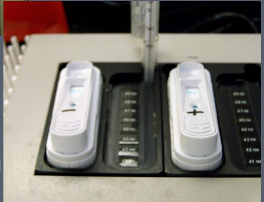
Devices labeled and placed on heater block
